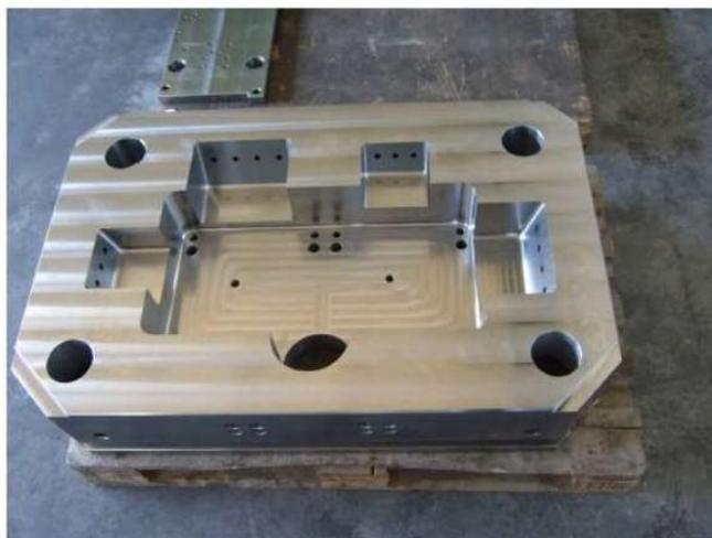
FRESATURA PORTASTAMPI PRESSOFUSIONE ALLUMINIO E ZAMA
